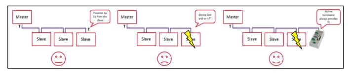
Additional note: Wherever a single wire enters a connector, the cable should always be wired into the 'incoming' port and not the outgoing, as the outgoing port is usually disconnected once the termination switch is enabled.
