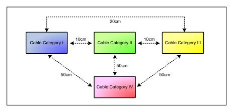
**Category I:** Fieldbus and LAN cables (E.g. PROFIBUS, ASi, Ethernet, etc.), shielded cables for digital data (E.g. Printer, RS232, etc.), shielded cables for low voltage (< 25 V) analogue and digital signals, low voltage power supply cables (< 60 V), coaxial signal cables.
