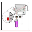
It is advisable to have Active Terminators installed at the ends of the segments so that the last device (usually responsible for providing the termination) can be replaced/allowed to fail, without affecting the rest of the network. A termination is a resistor circuit which requires 5V. A termination on a
